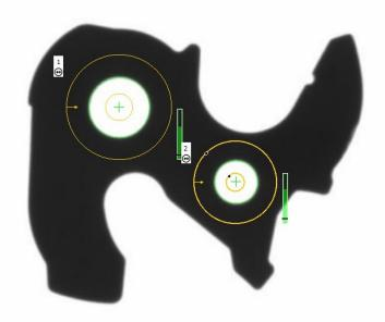
The Measuring Slide, Circle detector—also known as "Caliper, Circle" —precisely measures round features such as bores and washers. It reliably determines the diameter and center point of complete or partial circles. Perfect for metalworking, assembly, and handling tasks, it ensures accurate measurement of holes or differentiates between similar-looking parts like washers, Orings, and seals.
