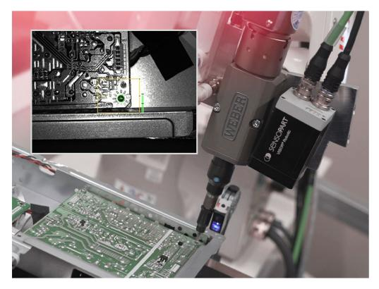
The new **Shape Find detector** enables fast and robust detection of geometric shapes such as rectangles, squares, and circles. VISOR® sensors can automatically identify all matching shapes within the image—or search specifically for user-defined parameters, such as a circle with a preset diameter in millimeters.
